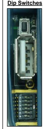
All Dip Switches must be set to the OFF position.
