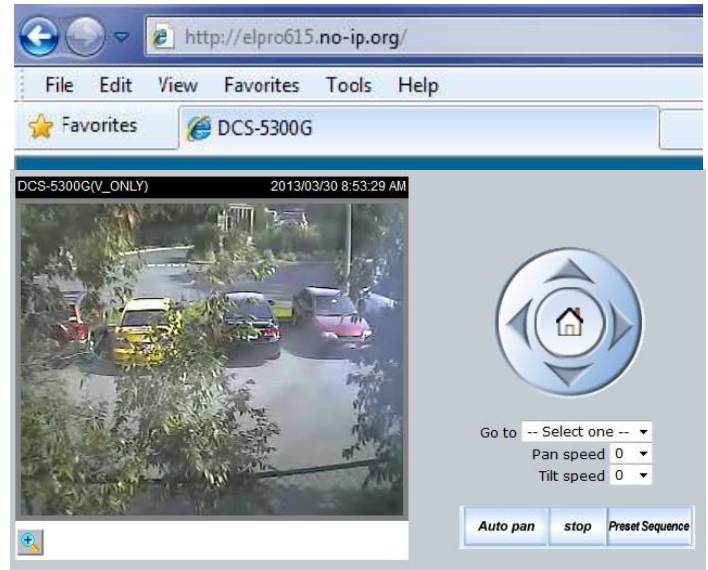
IP Mapping Table 2: Camera –Accessing a IP Web camera from a fixed internet IP address using Port 12080 from web browser.
