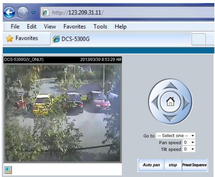
Accessing IP web camera via 615M-1 PPP IP Address
