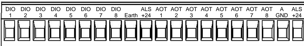
Figure 5-5: I/O terminal block for 115S-13.
