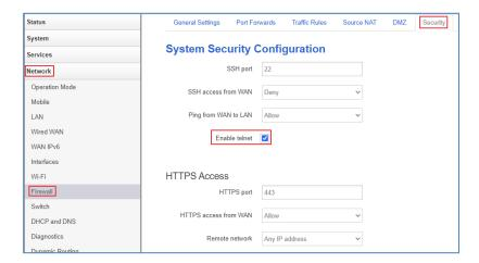
To do this use "Putty.exe" and connect to the LAN IP address via Telnet using Port 23. (see Screenshot)
