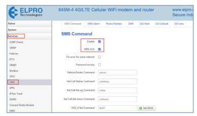
For Digital Inputs you will need to select the "SMS Alarms tab and then enable the "SMS Alarm" checkbox. Again press the "Save and Apply" button.
