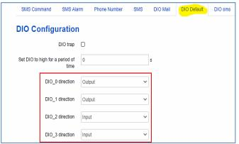
Elpro radio inputs are generally pulled high and are then activated when a Ground is switched to it. You will note in the screenshot that the DIO\_0-3 (Input 1-4) value for DIO\_2 & DIO\_3 are High (1) and will activate when the input is connected to GND and if you refreshed the Web page you would see the state change from "1" to "0" indicating the input is ON
