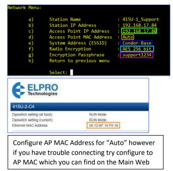
**Note:** The 415U-1 can connect to a 415U-X-C in any of the configured Networking Modes, i.e. Promesh, Fixed Links or Manual AP. Just need to make sure the ESSID matches the "Device Name" name.
