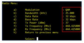
When all parameters have been setup, save the 415U-1 configuration by selecting "Save Config" from the previous menu options or by going back to the main menu and selecting option "g)" "Show/save configuration" and confirming "Y" when it asks to "Save Current Config? (y/n):"
